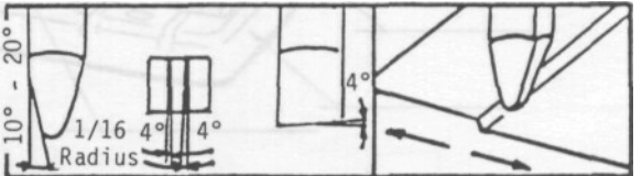
Round-nosed tool for bronze or brass
