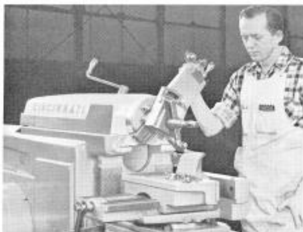
Shaping a short section of a press brake forming die.
